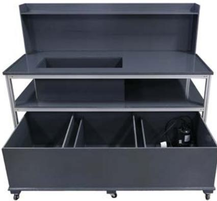
**How It Works-** Water that drains from the table into the sludge tank enters the first compartment. As the compartment fills the water travels through the baffling to the second and third compartment where it is pumped out.
