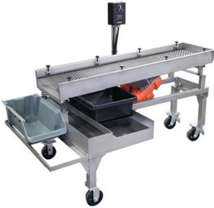
**How It works-** The PSA-1660 media separator utilizes two .15 hp shaker motors which are harmonized to create the vibration needed to separate media from parts. When the operator dumps media and parts onto the screen, media falls through the screen while parts stay on top. Screens are removable and come standard in 1/4 inch increments.
